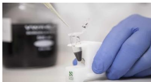
Fig. 6: A tube with magnetic beads.
