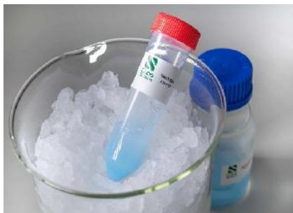
Fig.8: This batch spin is done on ice to prevent protein denaturation.
