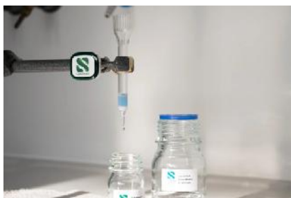
Fig. 9: A drip columns filled with our INDIGO agarose.
