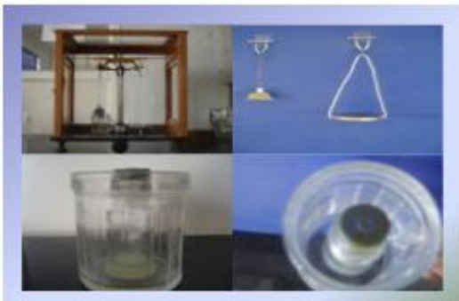
Fig 1: Bioadhesion strength apparatus
