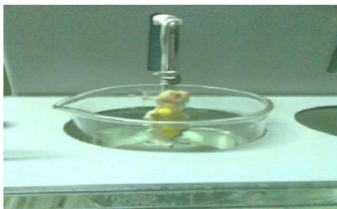
Fig 2: Ex vivo residence time measurement apparatus
