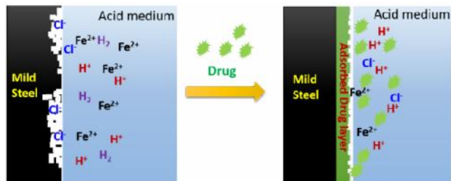
Figure 2: Typical action of a drug as a corrosion inhibitor in acidic medium
