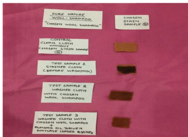
Figure 3: Washing results of stained woolen fabric pieces having hair color dye crème stain sample B (Garnier Nutrisse Black) with chosen wool shampoo named, Pure Nature WOLL-Shampoo and prepared bio-active almond oil driven BSANPs [20]
