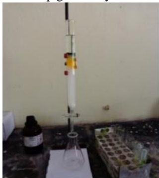
Figure 2: Isolation of pigments by Column Chromatography
