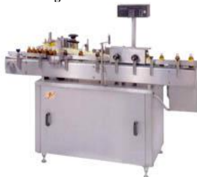
Figure 7: Automatic labeling machine
