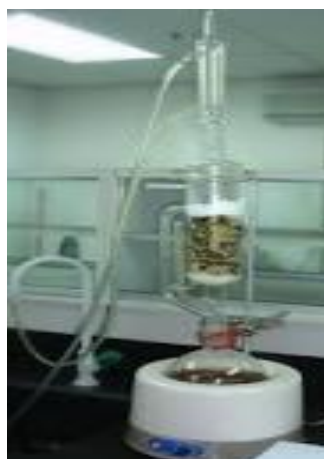
Figure 2: Methanol extract of Fegonia by sohxlet apparatus
