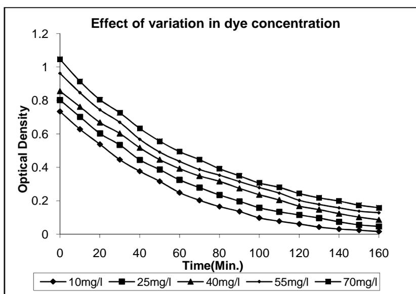
Figure 5. Effect of variation in dye concentration
