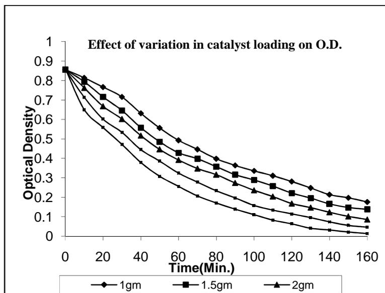
Figure 4. Effect of variation in catalyst loading on O.D
