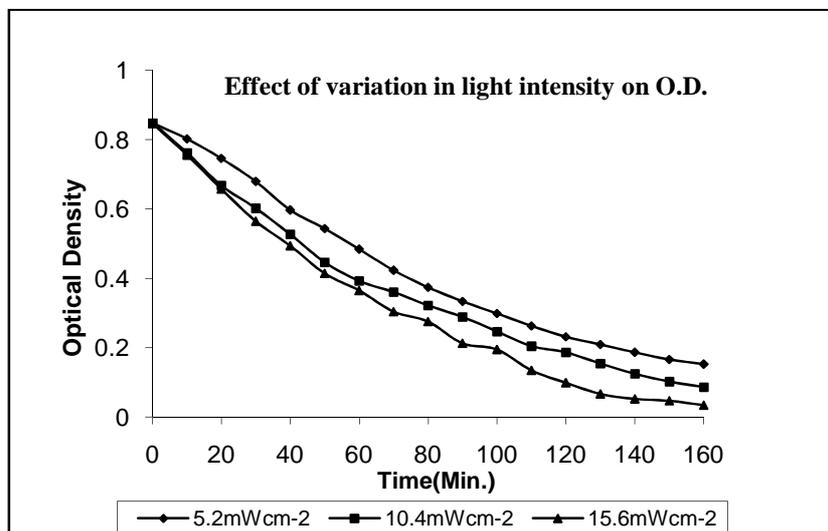
Figure 6. Effect of variation in light intensity on O.D
