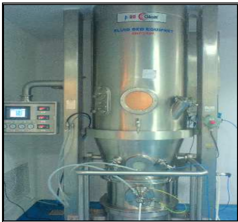
Figure No.8 Coating of Core Pellets
