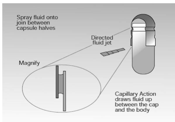
**Figure 3. Space between cap and body of the capsule spraying process to moisturize the hard gelatin capsules**
