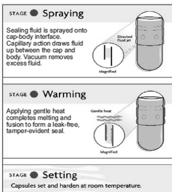
**Figure 2. Capsule sealing using a hydro-alcohol solution**
