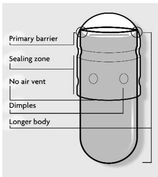
**Figure 1. Two-piece capsule for liquid fills**
