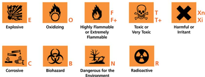
**Fig.8** Pictograms used in chemical hazards
