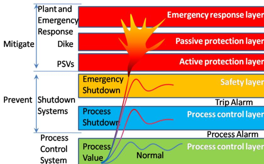
Fig. 9 Description of safety layer protection
