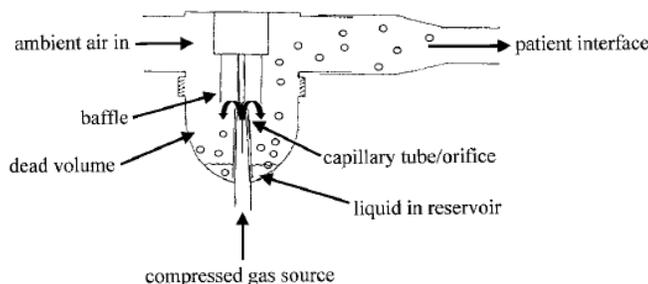
**Fig 7: Basic components of the design of pneumatic nebulizers**
