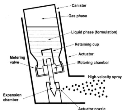
**Fig 9: Pressurized metered dose inhaler**
