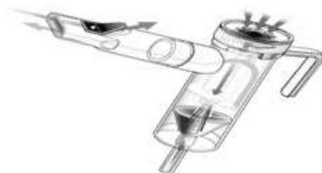
**Fig 8: Schematic representation of the function of a breath-enhanced nebulizer**
