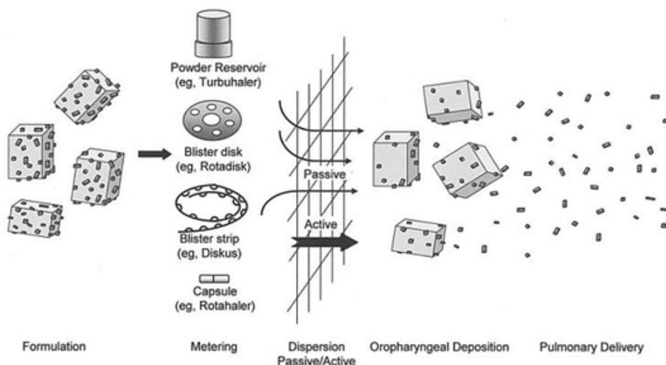
Figure 11: Principle of dry powder inhaler design
